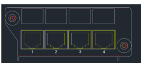
SM42R-004-00V: 4 Ports 10/100/1000 Base T combined with 4 socket 1000FX SFP
